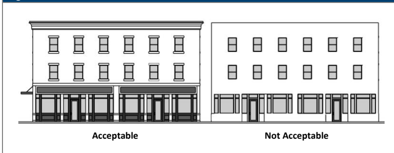
Figure 5-1-2-6: Horizontal and Vertical Articulation
