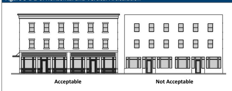
Figure 5-1-2-6: Horizontal and Vertical Articulation
