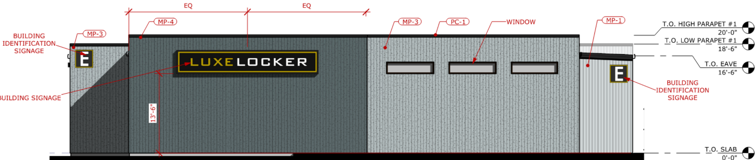
BUILDING E - SOUTH ELEVATION SCALE: 1/8" = 1'-0"
