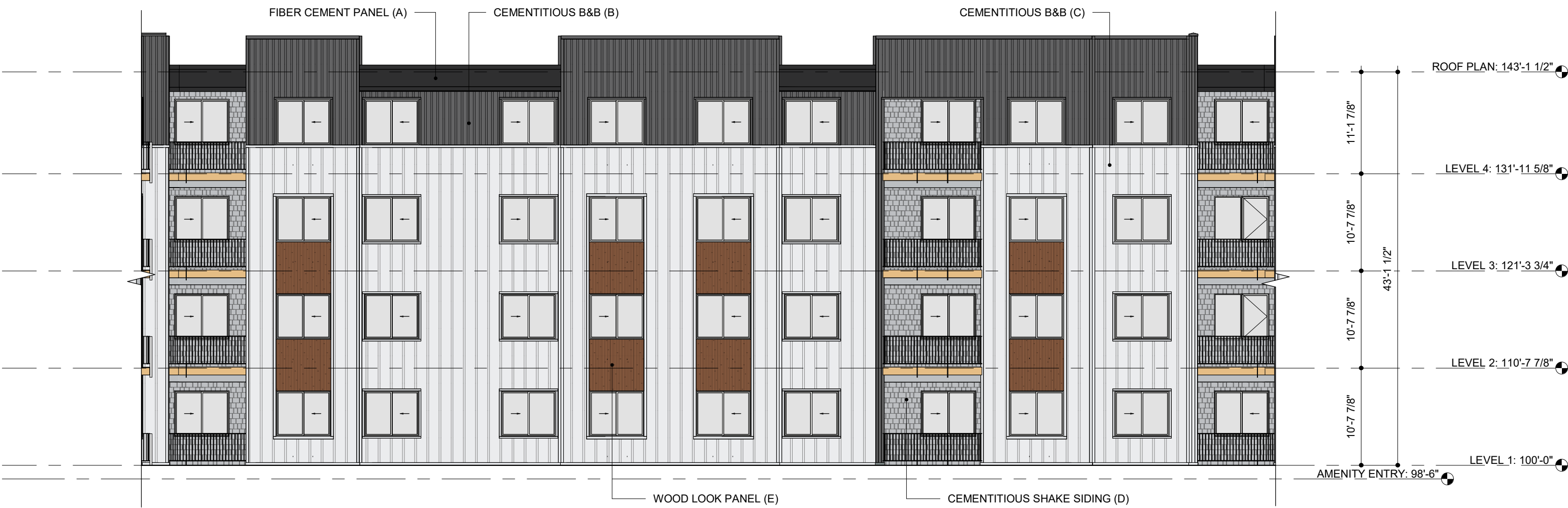
1 COURTYARD 02 SOUTH ELEVATION 3/32" = 1'-0"
