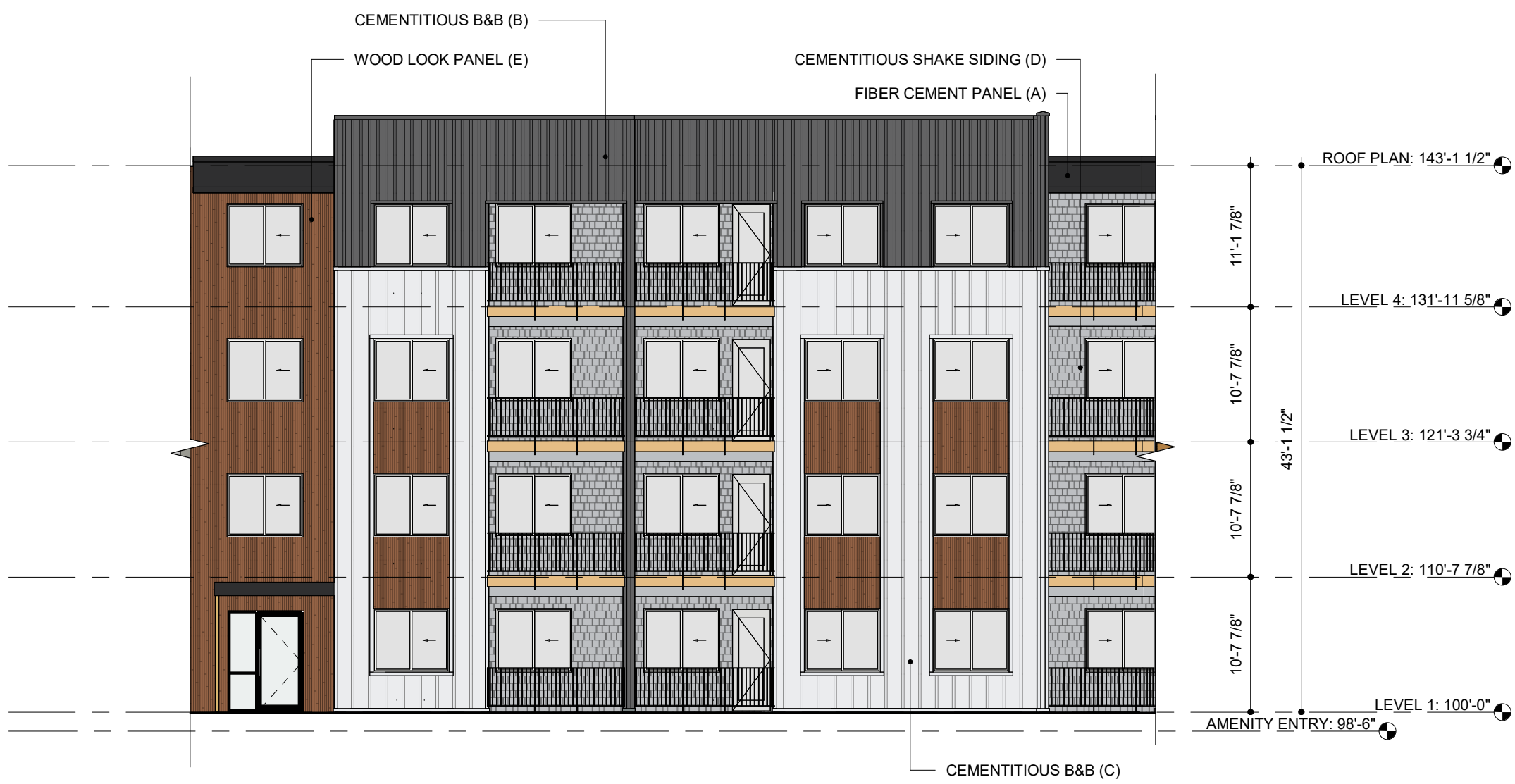
2 COURTYARD 02 EAST ELEVATION 3/32" = 1'-0"
