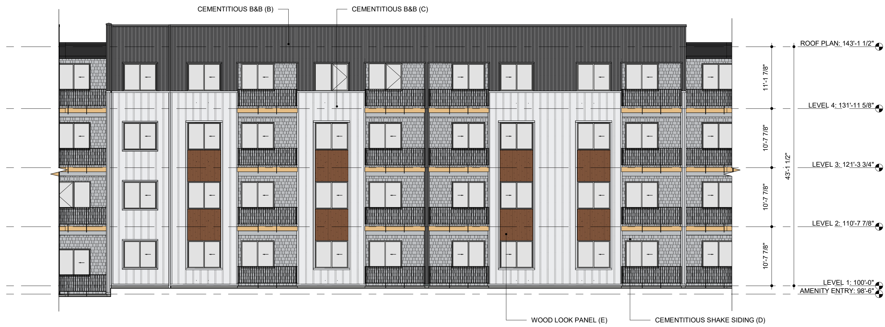
3 COURTYARD 01 SOUTH ELEVATION 3/32" = 1'-0"
