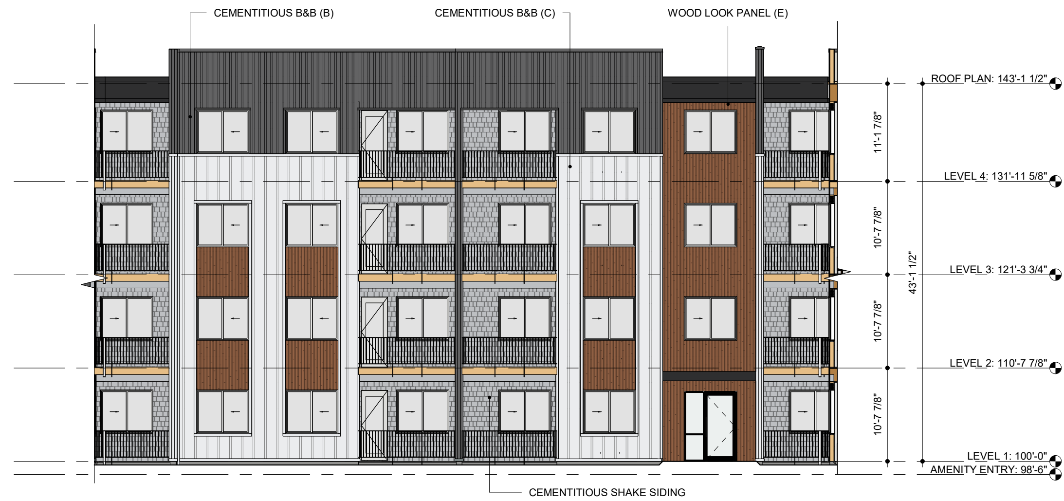
4 COURTYARD 01 WEST ELEVATION 3/32" = 1'-0"
