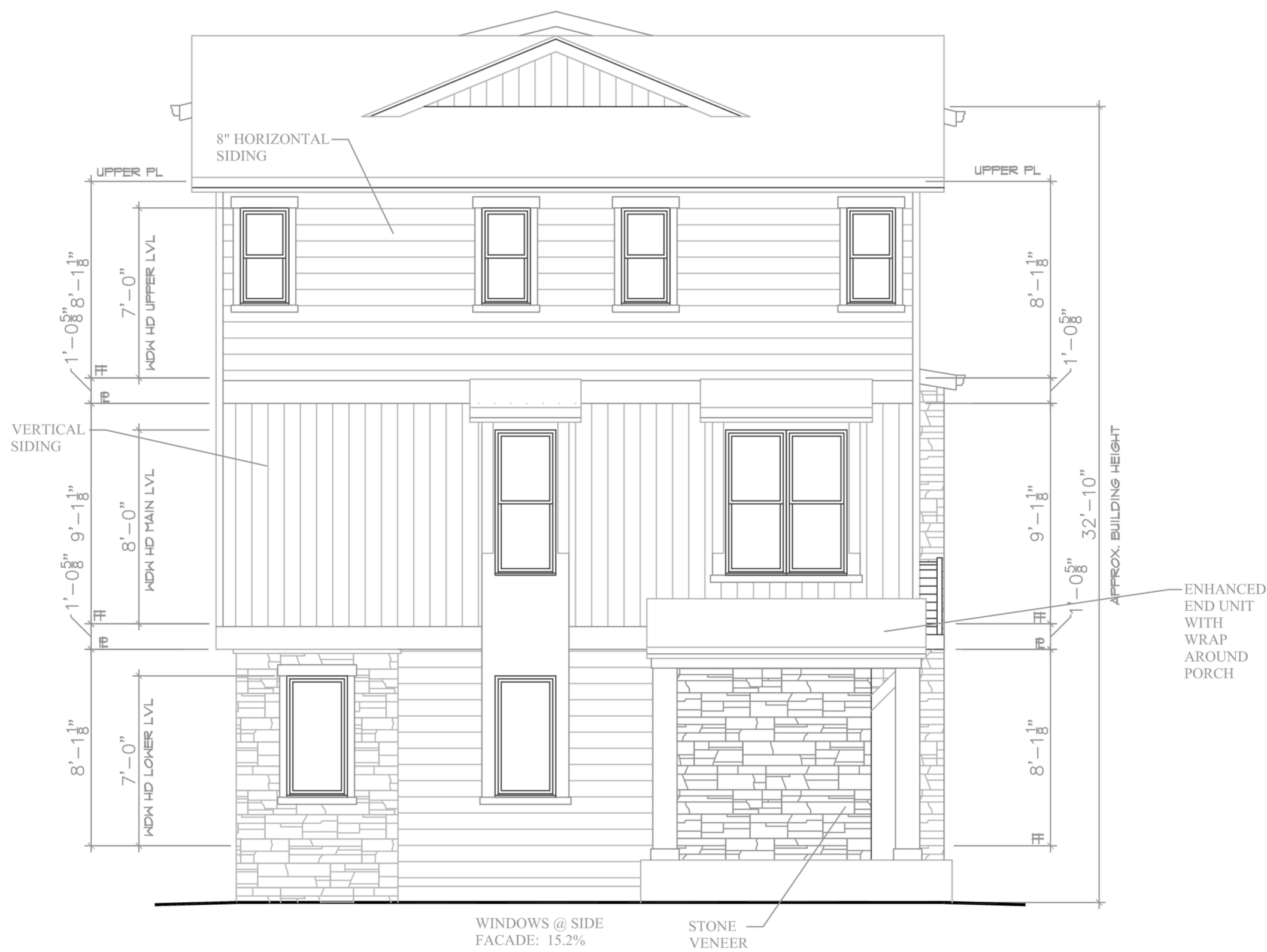
SIDE ELEVATION - ENHANCED END UNIT
