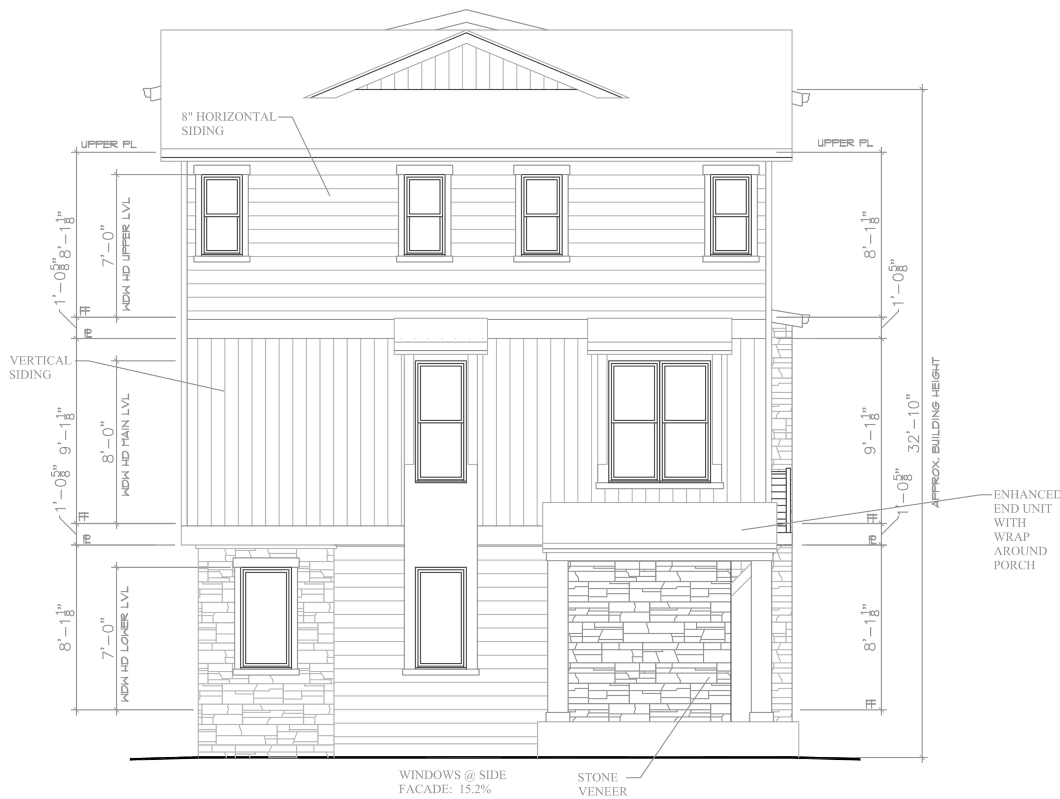
SIDE ELEVATION - ENHANCED END UNIT
