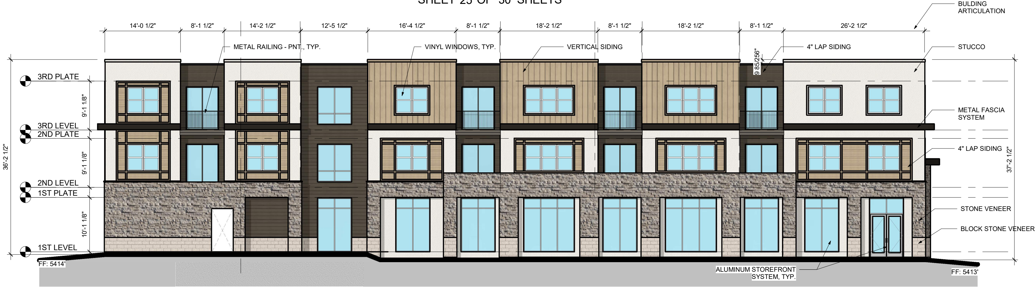
4 BUILDING 1-REAR ELEVATION (McINTYRE ST.) 3/32" = 1'-0"
