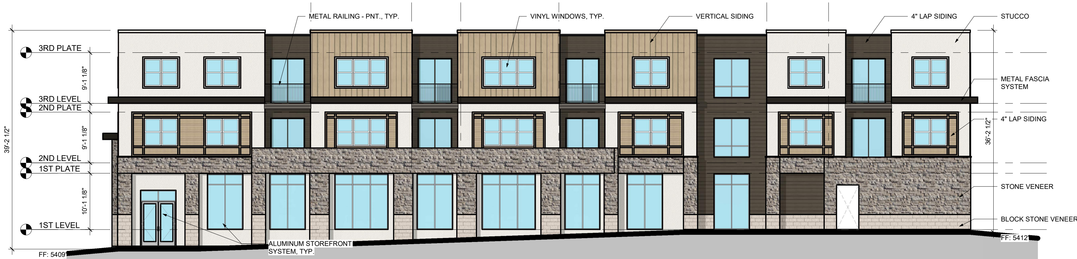
1 BLDG 2-REAR ELEVATION (McINTYRE ST.) 3/32" = 1'-0"
