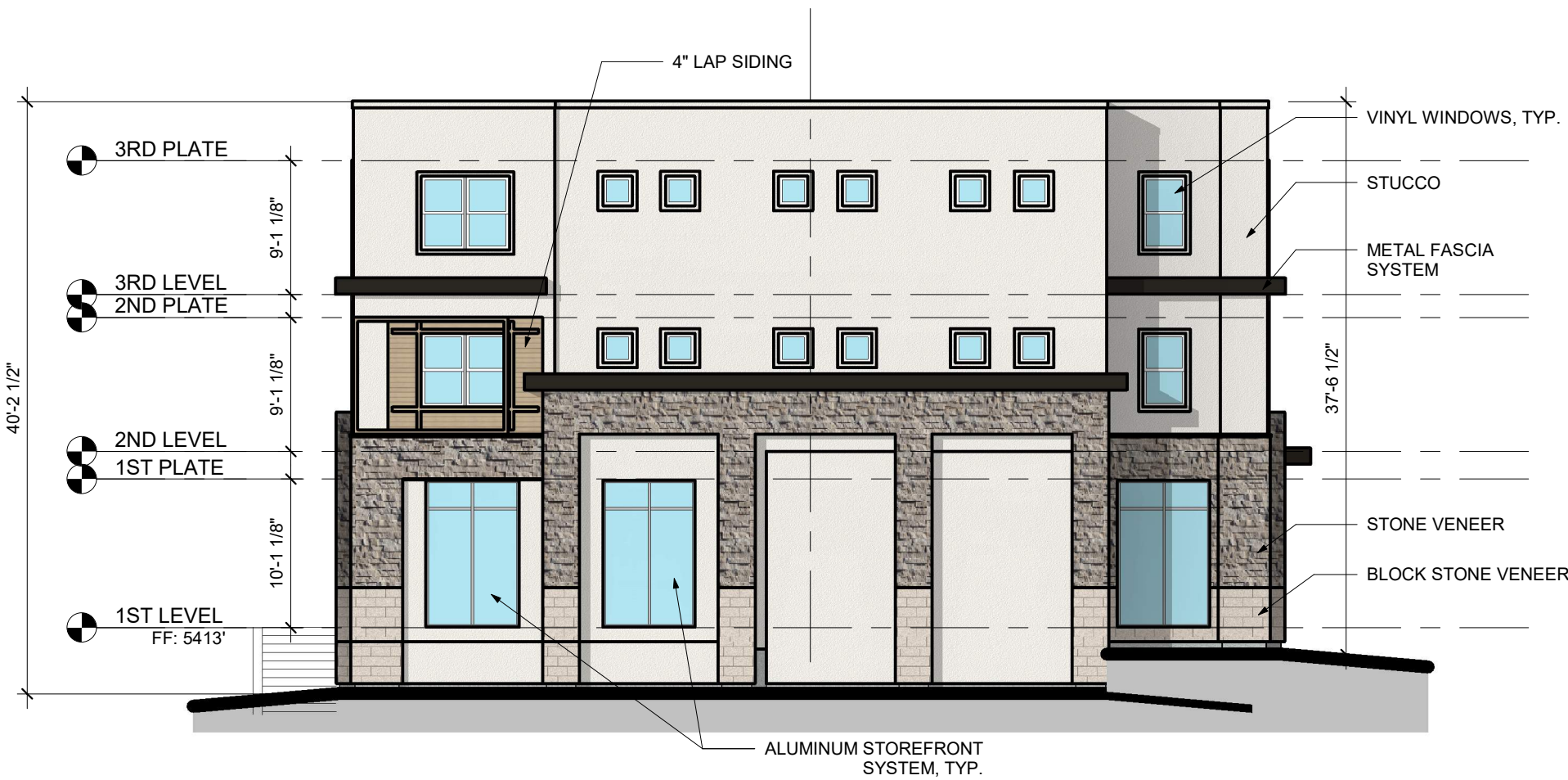
2 BUILDING 1-LEFT SIDE ELEVATION (W. 93RD PL.) 3/32" = 1'-0"
