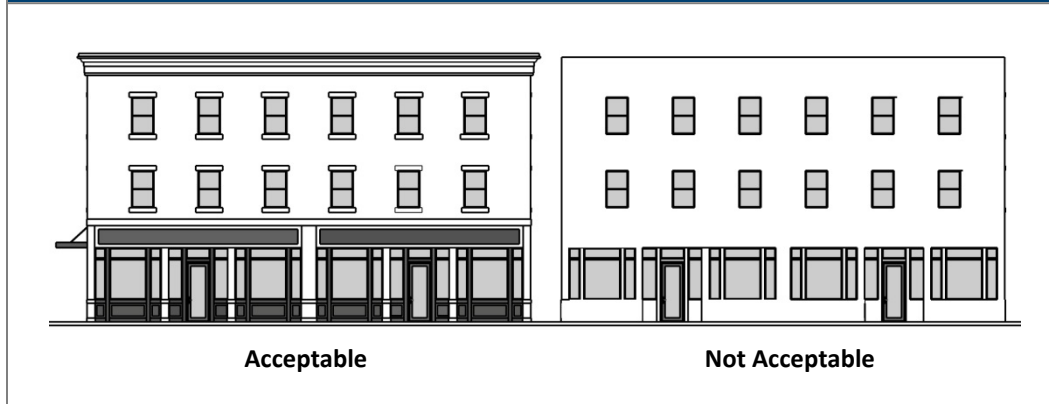
Figure 5-12-21-6: Horizontal and Vertical Articulation
