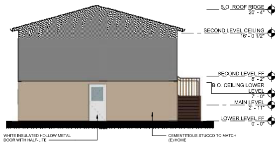
4 A-2 COLOR SOUTH ELEVATION OF ADDITION SCALE: 3/16" = 1'-0"
