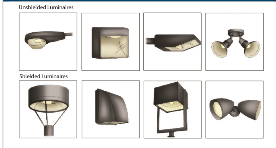
Figure 4-8-2-2: Light Fixtures Examples
