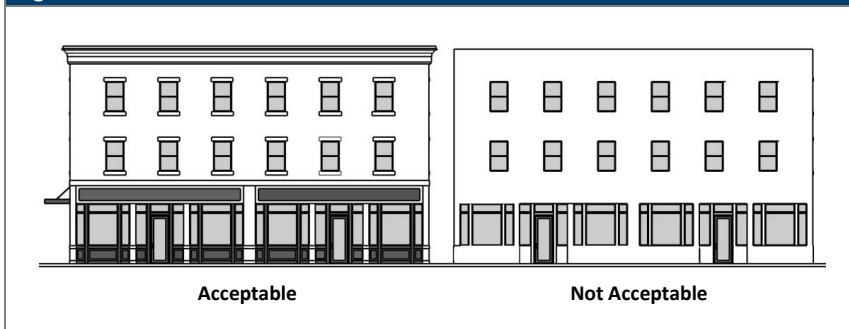
Figure 5-2-1-6: Horizontal and Vertical Articulation
