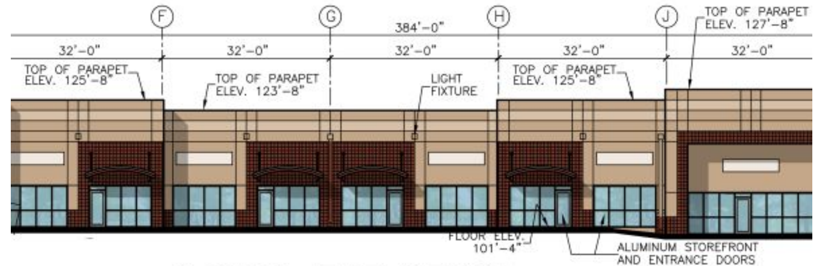
SOUTH ELEVATION (Facing 65th Way)
