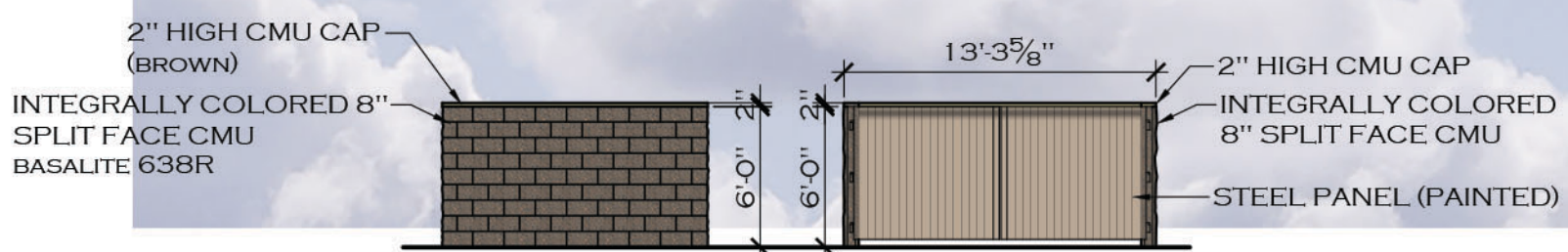
INTERIOR TRASH ENCLOSURE 6 SCALE: 1/8" = 1'-0"
