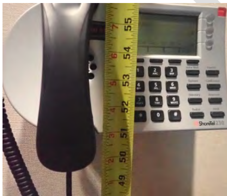
Figure 2.4.1.1(c) Typical Observation: Operable parts above required reach range: [ADA Standards 308. ]
