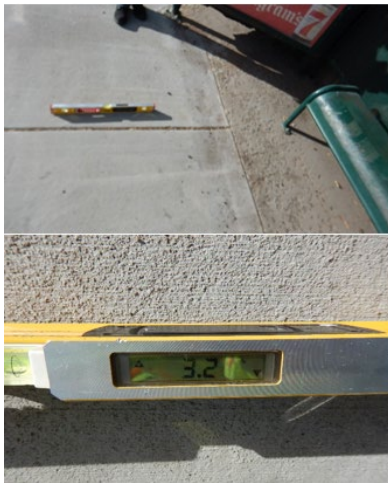
Figure 31 Measurement shows the slope at a bus stop, perpendicular to the street is 3.2%.
