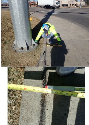
Figure 32 Data Collector measures obstructed reach distance to pedestrian control that is greater than 10 inches.
