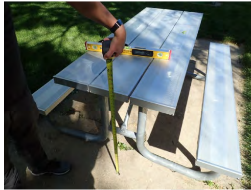
Figure 2.5.1.1(d) Typical Observation: Insufficient knee clearance at picnic table. [ADA Standards 306.3.3. ]
