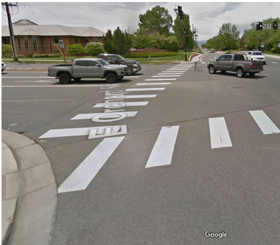
Figure 33 View of pedestrian street crossing at intersection across S. Holly Street at E. Orchard Road. The pedestrian walk interval was timed at 8 seconds to cross six traffic lanes.
