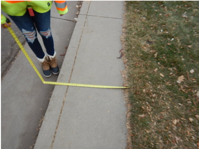
Figure 20 Data collector measures the width of a narrow sidewalk.
