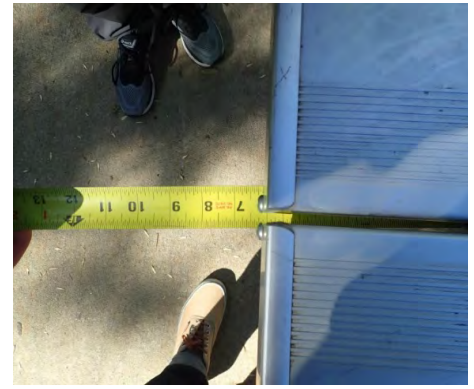
Figure 2.5.1.1(d) Typical Observation: Insufficient knee clearance at picnic table. [ADA Standards 306.3.3. ]
