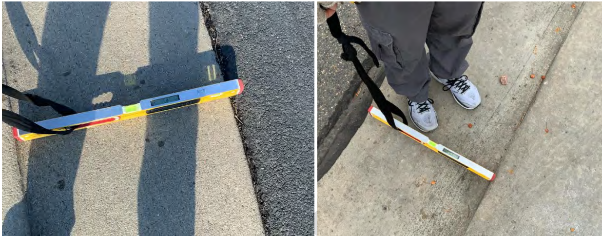
Figure 2.6.1.3(d) Typical Observation: Curb ramp has no turning space at top. [PROWAG R304.2.1. ]
