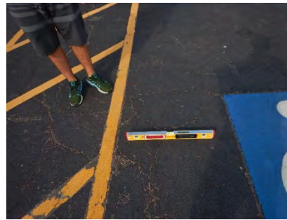
Figure 2.4.1.3(b) Typical Observation: Parking spaces with slopes too steep: [ADA Standards 502.4.]
