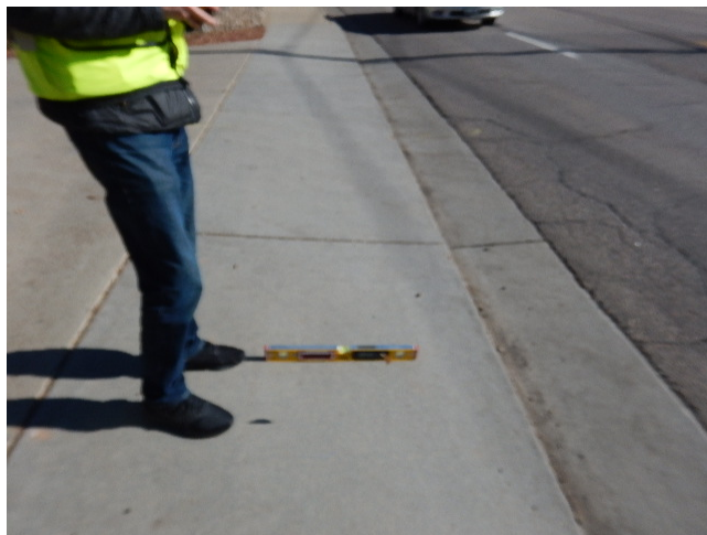
Figure 26 Data collector measuring the cross slope of sidewalk at driveway.
